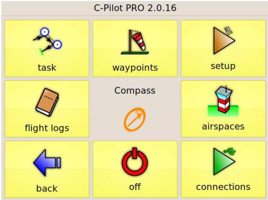
Figure 2. It shows up when you press the **C-Pilot PRO** button in the navigation page. After eight seconds it disappears automatically if you do not press any button; the navigation page will appear again.
