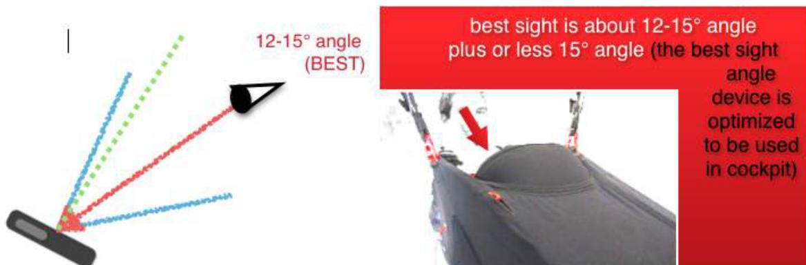
Figure 7: optimal in-flight position.
